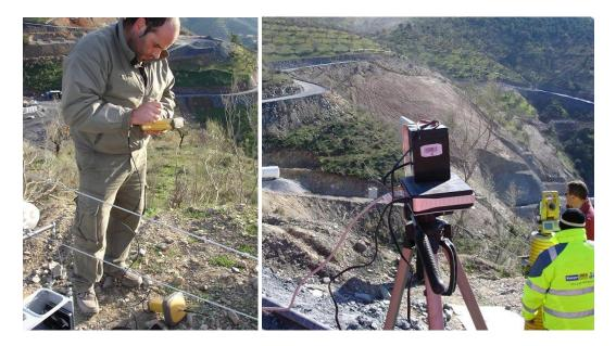
From a functional point of view, the system is fixed to a cable in such a way that it can move between two mounting points, in a blondin ropeway configuration, taking pictures and recording data of the position and orientation along the cable path. The system is connected to a remote PC, via a directional WiFi antenna (see Figure 2 (right)), for telemetry data logging and camera recording.
