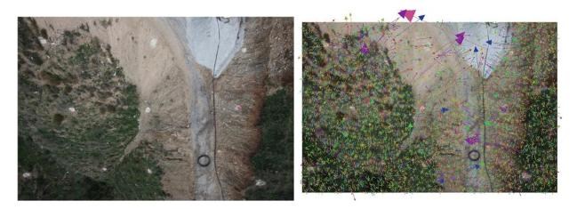
Figure 12. Single feature matching (left) and the complete set of matchings (right) in a given pair of images.
