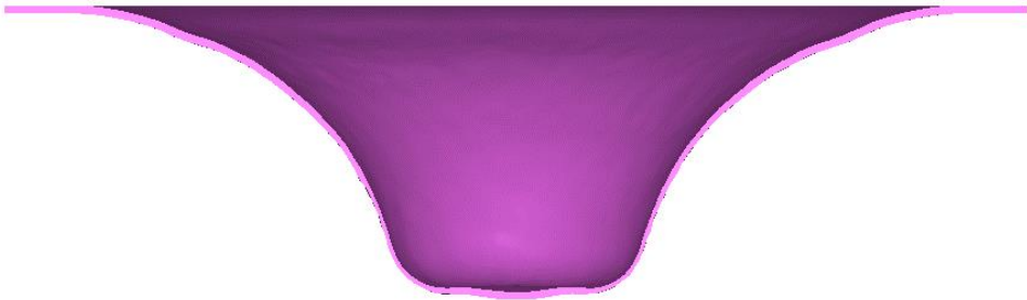
Figure 3.7 Final geometry of a SPIF formed AISI304 sheet with a 10 mm diameter tool
