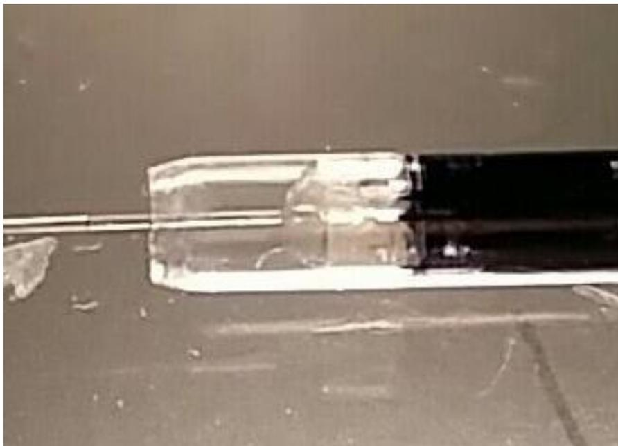
Figura 3-7. Protector Cap, SafeSpeed Device
