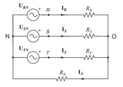
Fig. 1 Three-phase system with wye connection.
