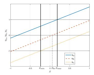
Fig. 1: Achievable phase levels for  $u_{\alpha}=1$  and  $u_{\beta}=0.5$  in 3-level converters.
