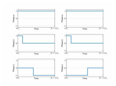
Fig. 4: Left and right: Two arbitrary sequences for  $u_a = 1$ ,  $u_b = 0.1289$ ,  $u_c = -0.5782$ . Sampling time is denoted by  $T_m$ .
