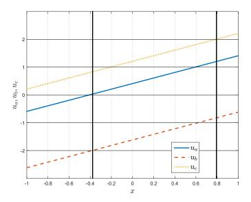
Fig. 2: Achievable phase levels for  $u_{\alpha} = 0.5$  and  $u_{\beta} = -2$  in five-level converters.
