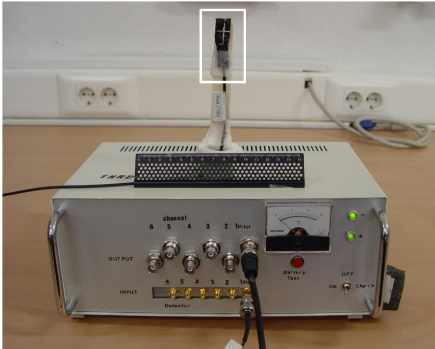
Figure 1. One of the TNRD detectors (marked with a white box) and associated six electronics channels.
