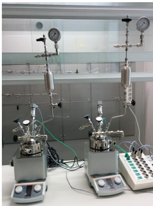
Figure 2-2.-Reaction system: batch reactors, heating plates, injection tanks and control
