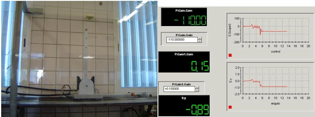
**Figure 6.** The linear actuator used as a base for the inverted pendulum (left) and a screen capture of the DSpace environment to perform control experiments using the linear actuator as a base for the inverted pendulum (right).
