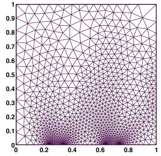
Figure 3: The final adapted mesh
