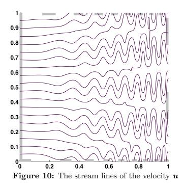
Such a velocity field is chosen in order to mimic a turbulent flow, and the corresponding stream lines are plotted in Figure 10. The Dirichlet boundary conditions on  $\Gamma_{-}$  are
