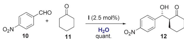
Scheme 4 Direct aldol reaction of p -nitrobenzaldehyde 10 and cyclohexanone 11 in water using nanocatalyst I .
