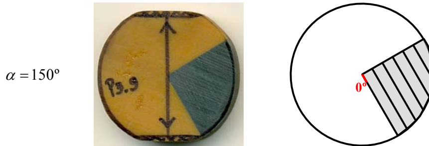
Fig. 6.24 – Tested samples and scheme of the failure path observed (static loading).
