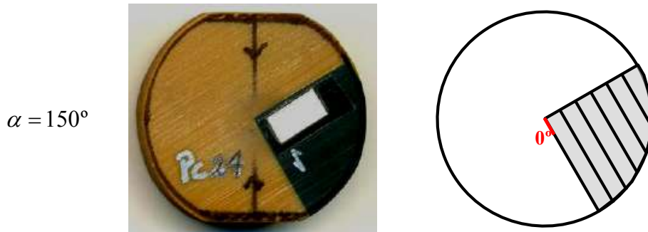
Fig. 7.15 – Tested samples and scheme of the failure path observed (fatigue loading).
