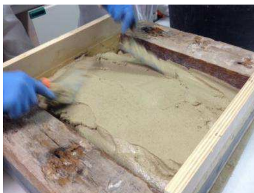
Fig. 8 “Pouring the mortar. a. Filling the upper side to the top to get a flat surface. b”. Source: the authors.
