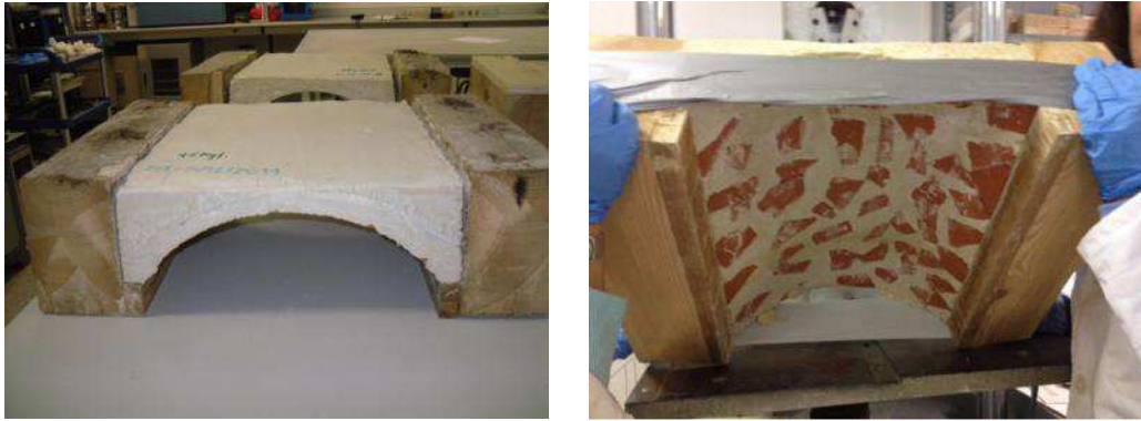
Fig. 9 “Finished piece after setting, and ready for burst testing”. Source: the authors.
