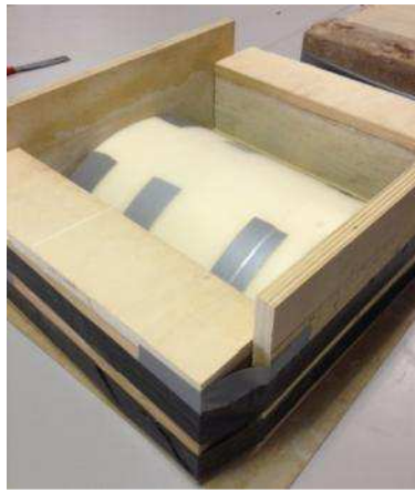
Fig. 6 “Location of the timber pieces and the mould to reproduce a real slab”. Source: the authors.
