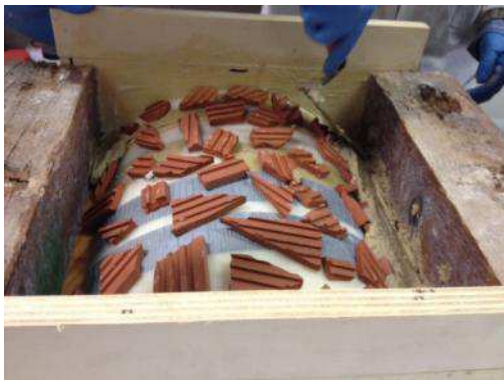
Fig. 7 “New piece production process. a. Placing the recycled ceramic demolition waste. b. Placing the fiberglass”. Source: the authors.
