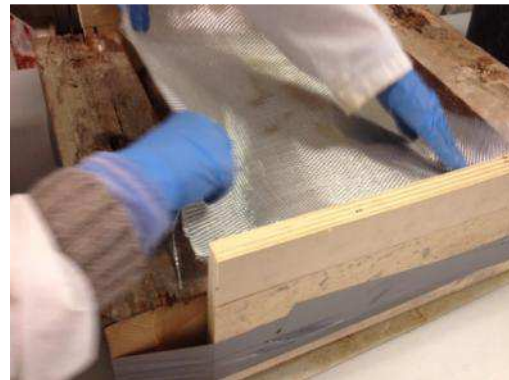
Fig. 7 “New piece production process. a. Placing the recycled ceramic demolition waste. b. Placing the fiberglass”. Source: the authors.
