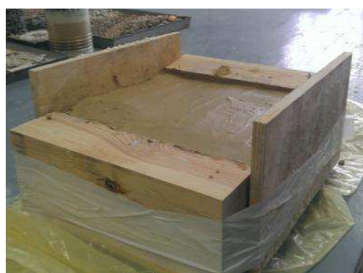
Fig. 8 “Pouring the mortar. a. Filling the upper side to the top to get a flat surface. b”. Source: the authors.
