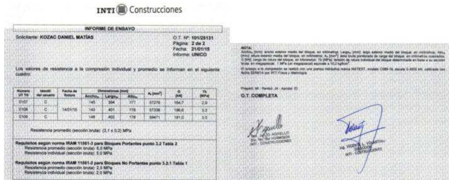
Fig. 8 “Compressive Strength tests performed in the INTI, Argentina”. Source: INTI
