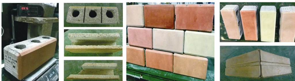
Fig. 7 "Different parts of the blocks system and color tests". Source: own elaboration
