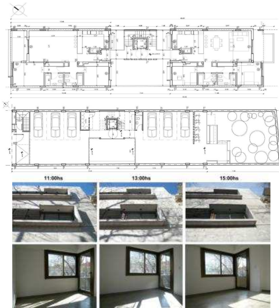
Fig. 1 “Ground Floor, 1 st and 2 nd Floorplan Aráoz plus Sunlight study”. Source: own elaboration
