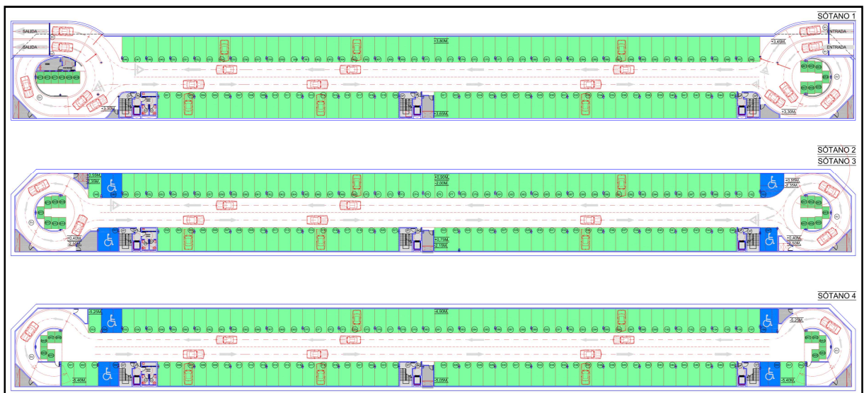
Fig. 3 "Underground parking. Distribution floors". Source: Author.
