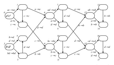
**Fig. 4.** A P system obtained from the bitonic sorting network of size 4 (Figure 3), in which each comparator has been replaced by a corresponding P system.
