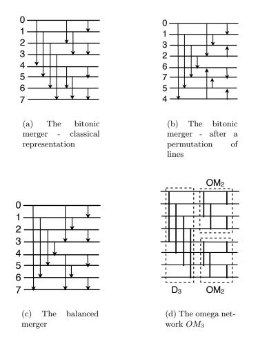
Fig. 3. The bitonic merger, the balanced merger, and the omega network of size 8
