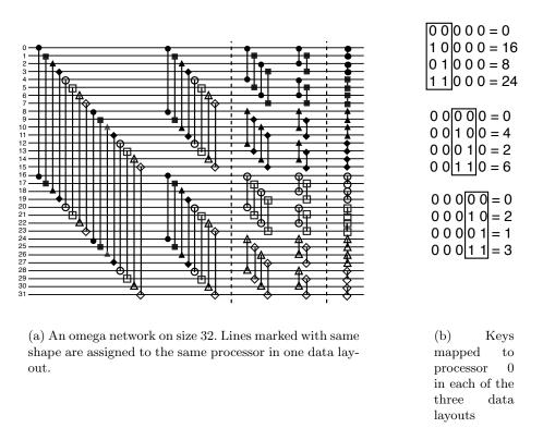
Fig. 4. Three data layouts for the omega network  $OM_5$ .
