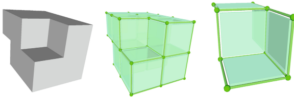
Fig. 2. Left: a binary volume. Center: its primal associated cubical complex. Right: its dual cubical complex
