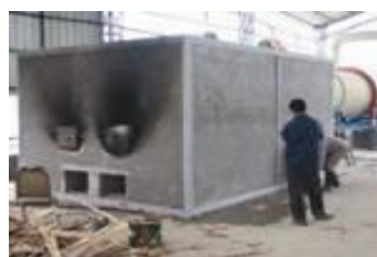
Crossing Wall Stove with multi-layer anti-air bricks
