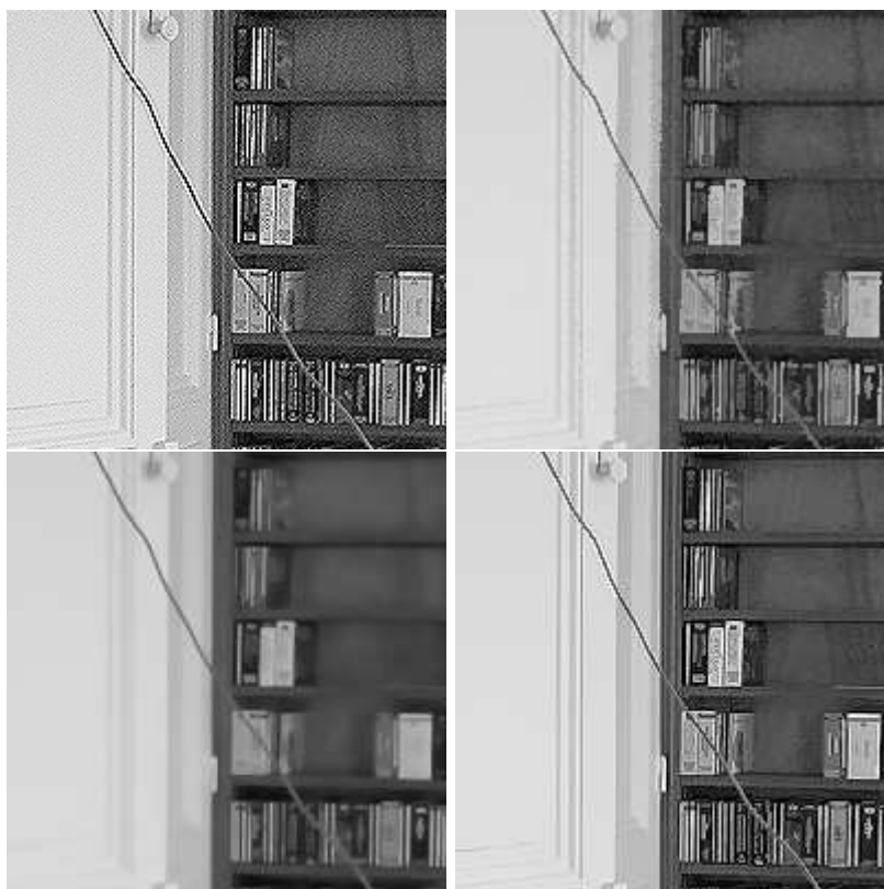
Figura 2: Comparison of different enhancement algorithms. From top to bottom and left to right: reverse heat equation ( t = 0,6 ), shock filter, the Perona-Malik equation and the non local reverse heat equation ( t = 0,6 ) with \lambda = 0,25 . The shock filter enhances noise and edge irregularities. The Perona-Malik equation enhances the main edges but blurs the rest of the image, thus losing many details.
