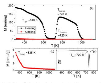
FIG. 2. (Color online) (a) Magnetization as a function of temperature at 0.3 T. (b) Magnetization curve for cooling process. (c) DSC scan for as-cast sample at 10 K/min.
