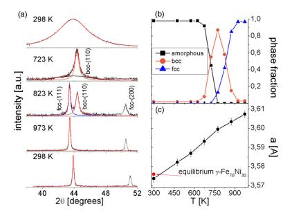
FIG. 1. (Color online) (a) *In situ* high-temperature x ray diffraction for some temperatures. (b) Temperature dependence of the phase fraction evolution. (c) Lattice parameter of the fcc-FeNi phase as a function of temperature.
