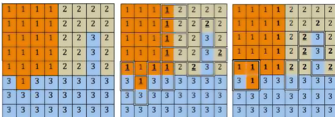
Fig. 2. C_0 (left): Original Image. C_1 (center): Some edge pixels have been marked. Only rules of type 1 have been used. C_2 (right): System has applied more rules of type 1 and one rule of type 2.
