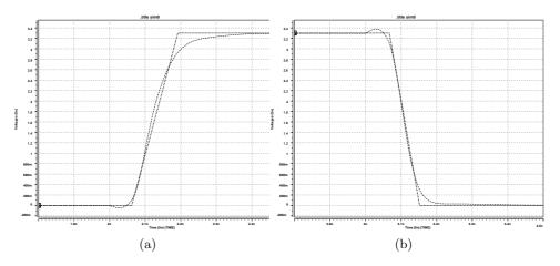
Fig. 1. Ramp approach method using 20%-80% criterion.
