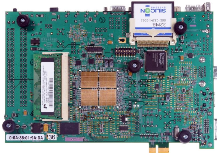
Imagen 5.6 – Vista trasera Virtex 5 FPGA Evaluation Platform LM505 [43]
