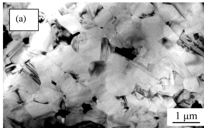
Fig. 4.28. SEM micrograph of 56% crept B 4 C ceramic SPS sintered at 1700 °C for 3 of the ultra-fine B 4 C powder prepared by high-energy ball-milling plus annealing.
