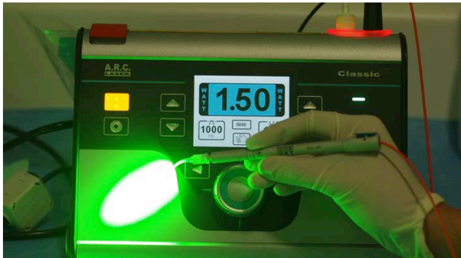
Figura 4.5 Láser de 532 nm o KTP .ARC MEDICAL LASER ®, modelo Classic Green Laser
