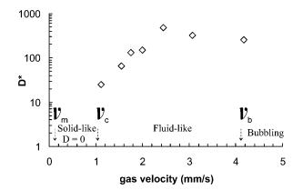
FIG. 4. Nondimensional diffusion coefficient  $[D^* = D/(v_g d_p)]$  obtained from the fit between experimental and theoretical values of magenta toner concentration as a function of gas velocity.
