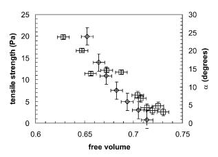
FIG. 2. Tensile strength  $(\diamondsuit)$  and angle of avalanche  $(\Box)$  as a function of the powder free volume for the magenta toner.
