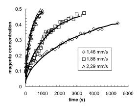
FIG. 3. Experimental values of the magenta toner concentration over the initially yellow side and theoretical curves assuming a Fickian diffusion process for different values of the gas velocity.
