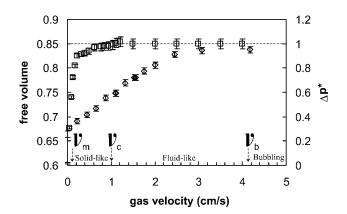
FIG. 1. Free volume ( $\diamond$ ) of the powder bed (a mixture of 50% magenta toner and 50% yellow toner) and gas pressure drop ( $\Delta p^*$ ) normalized to the bed weight per unit area ( $\Box$ ) as a function of gas velocity.
