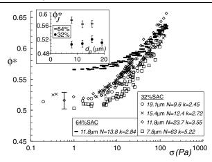
FIG. 4. Cluster volume fraction  $\phi^* = \phi k^3/N$  as a function of the normal stress for the set of experimental toners of Fig. 3. Also plotted are data for the 11.8  $\mu$ m particle size, 64% SAC experimental toner. The error bar is the typical indeterminacy in  $\phi^*$ . The inset shows the cluster volume fraction at the jamming transition  $\phi_I^*$  as a function of particle size.
