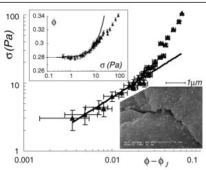
FIG. 2. Normal stress as a function of the increment of the particle volume fraction beyond the jamming threshold ( $\sigma > 0$ ) for Canon CLC700 powder. Insets: (top)  $\phi$  as a function of  $\sigma$  showing  $\phi_J \simeq 0.28$ ; (bottom) SEM micrograph of a toner particle surface with 64% SAC. The continuous line corresponds to the power law  $\sigma \simeq 271(\phi - \phi_J)^{0.824}$  Pa that is fitted to the data in the range  $\sigma < \simeq 15$  Pa.
