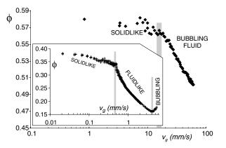
FIG. 1. Particle volume fraction of noncohesive PMMA beads  $(d_p = 200 \ \mu\text{m})$  in the fluidized bed as a function of the gas velocity. The inset shows the data for a cohesive powder  $(d_p = 11.8 \ \mu\text{m}, 64\% \text{ SAC})$ . The jamming transitions are indicated by vertical bars.
