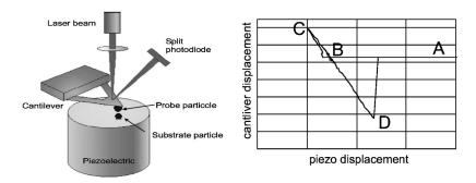
FIG. 8. Experimental setup for the measurement of interparticle forces with an atomic force microscope and a typical load-unload curve.
