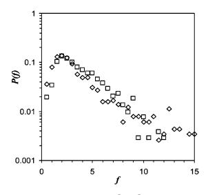
FIG. 10. Probability distribution [P(f)] of the adhesion force measured from the AFM normalized to the estimated adhesion force from the bulk stresses (f). Powder with 0.4 wt. % of additive (boxes). Powder with 0.05 wt. % of additive (diamonds).
