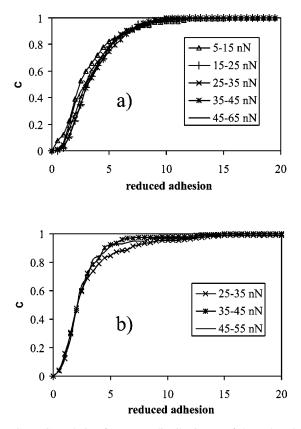
FIG. 9. Cumulative frequency distribution C of the reduced adhesion for different ranges of load force (indicated in the inset). (a) powder with 0.4% of additive, (b) powder with 0.05 wt.% of additive.
