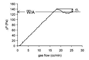
FIG. 4. Typical curve for the pressure drop across the powder bed vs gas flow (xerographic toner with particle size 12.7  $\mu$ m, 0.4% by weight of flow additive). The overshoot of the pressure drop beyond the weight per unit area of the bed (~130 Pa) is taken as the tensile strength of the powder ( $\sigma_t \approx 10$  Pa).
