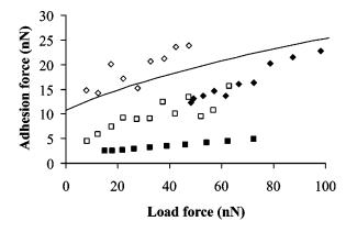
FIG. 7. Average (median value) adhesion vs load force measured from the AFM (void symbols) and estimated from bulk stresses (solid symbols). Powder with 0.4 wt. % of additive (boxes). Powder with 0.05 wt. % of additive (diamonds). The continuous line represents the theoretical prediction by the MP model [Eq. (13)] for a contact between polymer particles.
