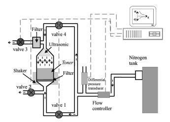
FIG. 3. Experimental setup for the measurement of the tensile strength as a function of the consolidation stress.
