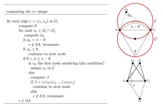
Table 1: Algorithm for computing the  $\alpha$ -shape. Note that all the computations require only local information. The angles denoted as illustrated in the figures on the right
