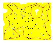
Figure 1:  $\alpha$ -shape with parameter  $r_c/2$  for a set of points in  $\mathbb{R}^2$  computed using algorithm in Table 1. The shaded region is the union of balls of radius  $r_c/2$  centered at each point.
