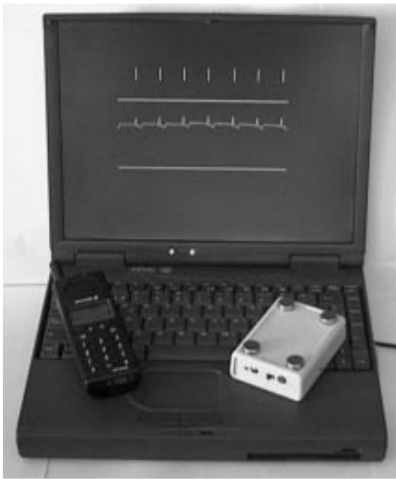
Figure 2: Portable electrocardiograph equipment (white box) and ECG signal transmitted to a laptop
