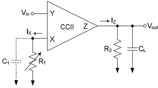
Fig. 4 Programmable Gain Voltage Amplifier using CCII
