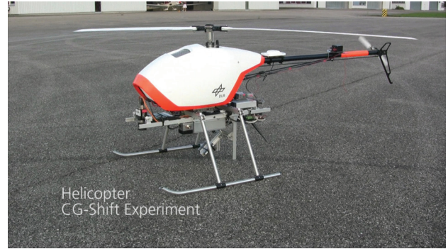
Figure 12. Experimental platform with pendulum for displacement of the helicopter CoG.
