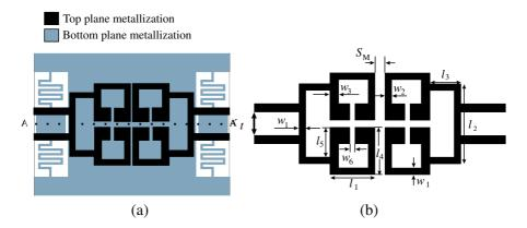
Figure 7. (a) Layout of the proposed dual-band filter with the common-mode suppression stages. (b) Final dimensions of the resonators: s = 1 mm,  $s_M = 0.2 \text{ mm}$ , t = 3.2 mm,  $w_1 = 0.3 \text{ mm}$ ,  $w_2 = 0.3 \text{ mm}$ ,  $w_3 = 0.6 \text{ mm}$ ,  $w_4 = 2 \text{ mm}$ ,  $w_5 = 2.5 \text{ mm}$ ,  $w_6 = 0.2 \text{ mm}$ ,  $l_1 = 4.2 \text{ mm}$ ,  $l_2 = 10.4 \text{ mm}$ ,  $l_3 = 1.3 \text{ mm}$ ,  $l_4 = 5.3 \text{ mm}$ .
