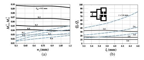
**Figure 8.** (a) Coupling coefficients for the first  $(M_{1,2}^{(1)}:$  solid lines) and second  $(M_{1,2}^{(2)}:$  dashed lines) bands as a function of the ratio  $w_3/w_2$ using  $s_M$  as parameter. (b) External quality factor at the first  $(Q_1:$ solid lines) and second  $(Q_2:$  dashed lines) resonance frequencies versus  $l_5$  using t as parameter. The other geometrical dimensions have the values show in Fig. 7.
