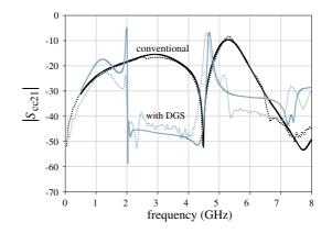
Figure 10. Common-mode insertion losses of the proposed filter. [Solid lines]: simulation results, [dotted lines]: measurements. Black curves are for the filter without common-mode suppression sections.
