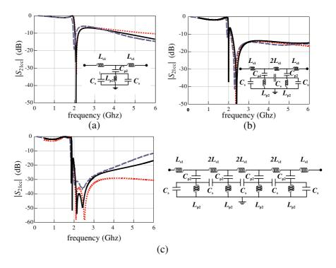
**Figure 3.** Full-wave simulated (solid black lines) and measured (blue dashed lines) common-mode responses for: (a) a single unit cell, (b) two cascaded unit cells, (c) four cascaded unit cells. Equivalent circuits and their predicted behavior (red dotted lines) are included.
