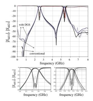
**Figure 9.** Differential-mode response of the proposed dual-band filter. [Solid lines]: simulation results, [dotted lines]: measurements. Black curves are for the filter without common-mode suppression section.
