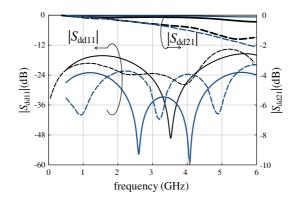
**Figure 4.** Measured (dashed lines) and calculated (solid lines) differential mode insertion  $(|S_{dd21}|)$  and return  $(|S_{dd11}|)$  losses of four cascaded cells of the proposed structure (black curves). The measured (dashed) and calculated (solid) response for a conventional pair of coupled lines (blue curves) has been included for comparison.
