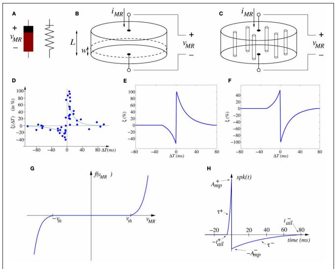
**FIGURE 3 | (A)** Memristor asymmetric symbols. **(B)** Illustration of moving wall model describing memristor operation as two variable resistors in series. **(C)** Illustration of filament formation/annihilation model describing memristor operation as two variable resistances in parallel. **(D)** Experimentally measured STDP function  $\xi(\Delta T)$  on
