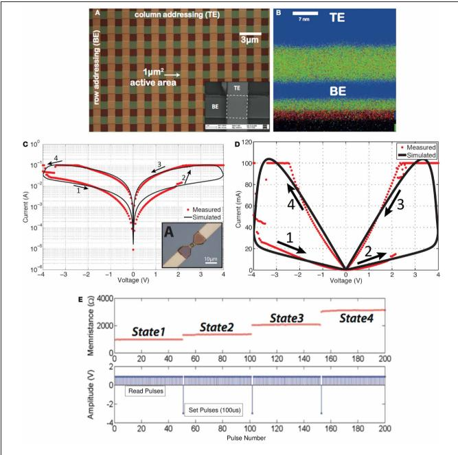
FIGURE 2 | Solid-state  $TiO_2$ -based memristors fabricated at Imperial College London. (A) Microphotograph of a memristor cross-bar array, with a close-up SEM illustration of a single cell appearing in the inset of (A). (B) CHEMI-STEM map of a lamella cross-section of one of the devices shown in (A): blue denotes Pt (top and bottom electrodes) while green and red correspond to Ti and  $O_2$  species (Prodromakis et al., 2012a). (C) Simulated and measured pinched hysteresis I-V characteristics
