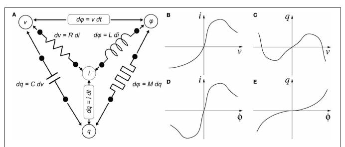
FIGURE 1 | Four variables of circuit theory linked by six mathematical relations consisting of the functional relationships of the four passive circuit elements, Faradays law of induction and the definition of electric current. (A) Chua's symmetry argument and (B–E) descriptions of the four canonical two-terminal devices. (B) A resistor is defined by a static
