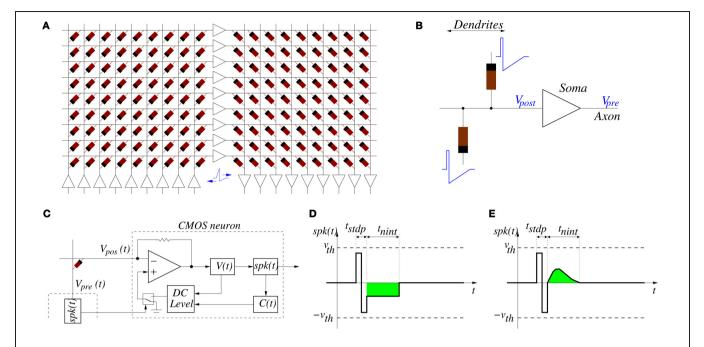
**FIGURE 5 | (A)** Example of memristors and CMOS neuron circuits arrangement for achieving STDP learning: feed-forward neural system with three layers of neurons and two fully connecting synapse crossbars. **(B)** Details of parts around one post-synaptic neuron. While a neuron is silent, it sets a constant DC voltage at its input  $(V_{\rm post})$  and output  $(V_{\rm pre})$  nodes. When a neuron is sending a spike, it sets a
