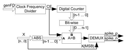
Figure 6. Reverse Bitwise Synthetic Spikes Generator internal blocks.
