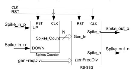
Figure 10. Spikes Integrate & Generate block diagram.
