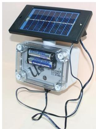
These nodes were designed as a general device system that allows distributed and collaborative data processing over the network, using IEEE 802.15.4 2.4 GHz radio transceivers.
