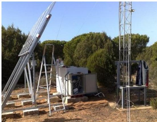
Each communication tower provides a local wired network, Wi-Fi, and a wired datalogger, which allow it to deploy sensors in the surroundings of these towers. Moreover, these towers provide power energy to wired sensors by solar panels.
