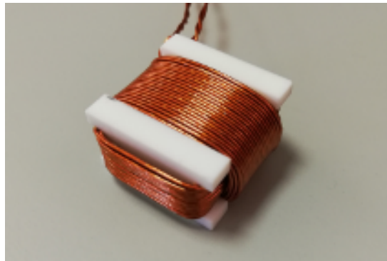
FIG. 3: 2D magnetic probe for SMART. The sensor is 25 x 25 x 15 mm in size and is wound using Kapton insulated copper wire of 0.4 mm in diameter on a Macor former.
