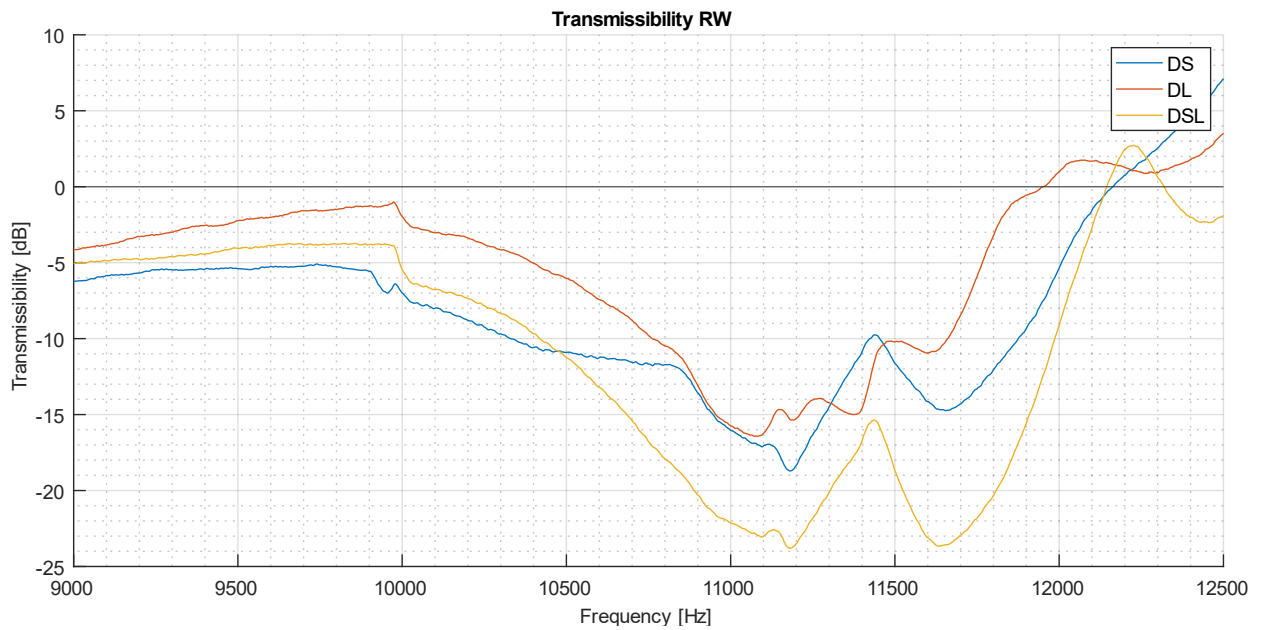
Figure 5.6: transmissibility of the reflected wave in all specimens at around 11,000 Hz
