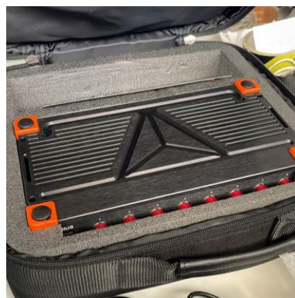
Figure 3.11: SIRIUS-8xACC-8xAO acquisition board
