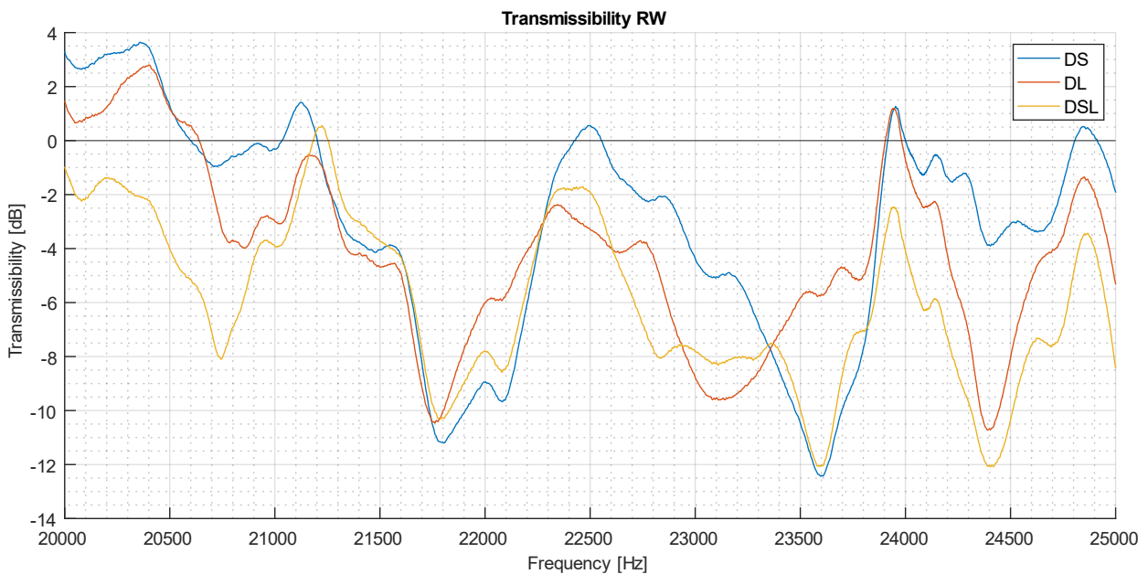
Figure 5.9: transmissibility of the reflected wave in all specimens between 20,000 Hz and 25,000 Hz
