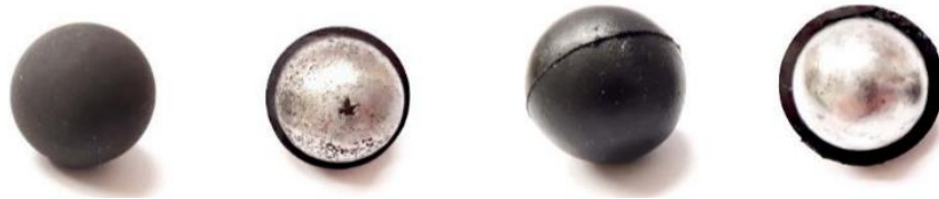
Figure 2.1: inclusions used in the thesis “Metaconcrete: Experimental Investigation on Samples with Inhomogeneous Inclusions” [2]
