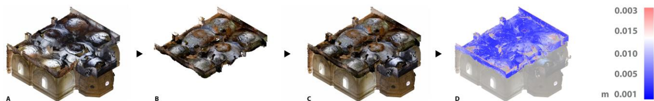
Fig. 3: (a) Scanner cloud, (b) photogrammetric cloud, (c) combined cloud and (d) deviation map
