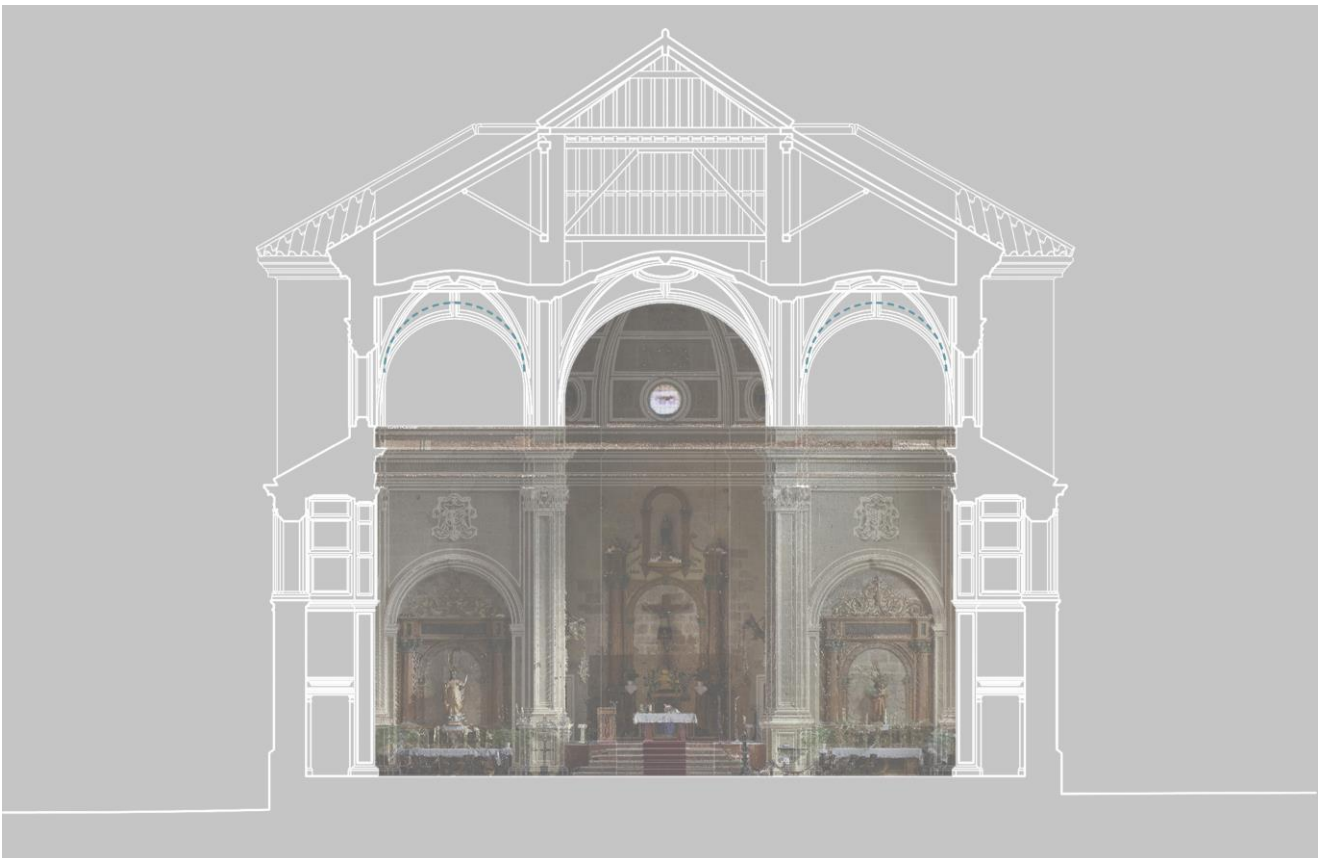
Fig. 15: Cross-section of the church looking towards the north end: wall ribs with the corrected height (in blue) and triumphal front (superimposed point cloud)
