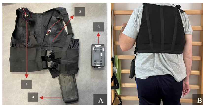
Figure 1. (A) Walking Aid ReMoD V5.0 Type 1 (vest and device). 1: Connection cables that transmit the signals, and where the electrodes are plugged in (the electrodes are then placed on the patient's skin to provide stimulation). 2: Sensors integrated in the vest. 3: ReMoD V5.0 Type 1 control unit device, which provides the electrical stimulus (it features multiple buttons for setting and controlling the signal intensity). 4: Pouch for storing the device while it is in use. (B) Case 1 standing autonomously with the ReMoD vest in a session.
