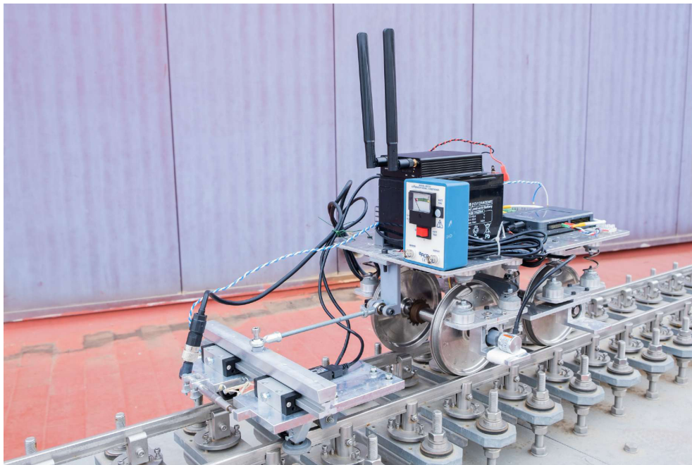
Fig. 7. Instrumented axle and propelling vehicle on the scaled track
