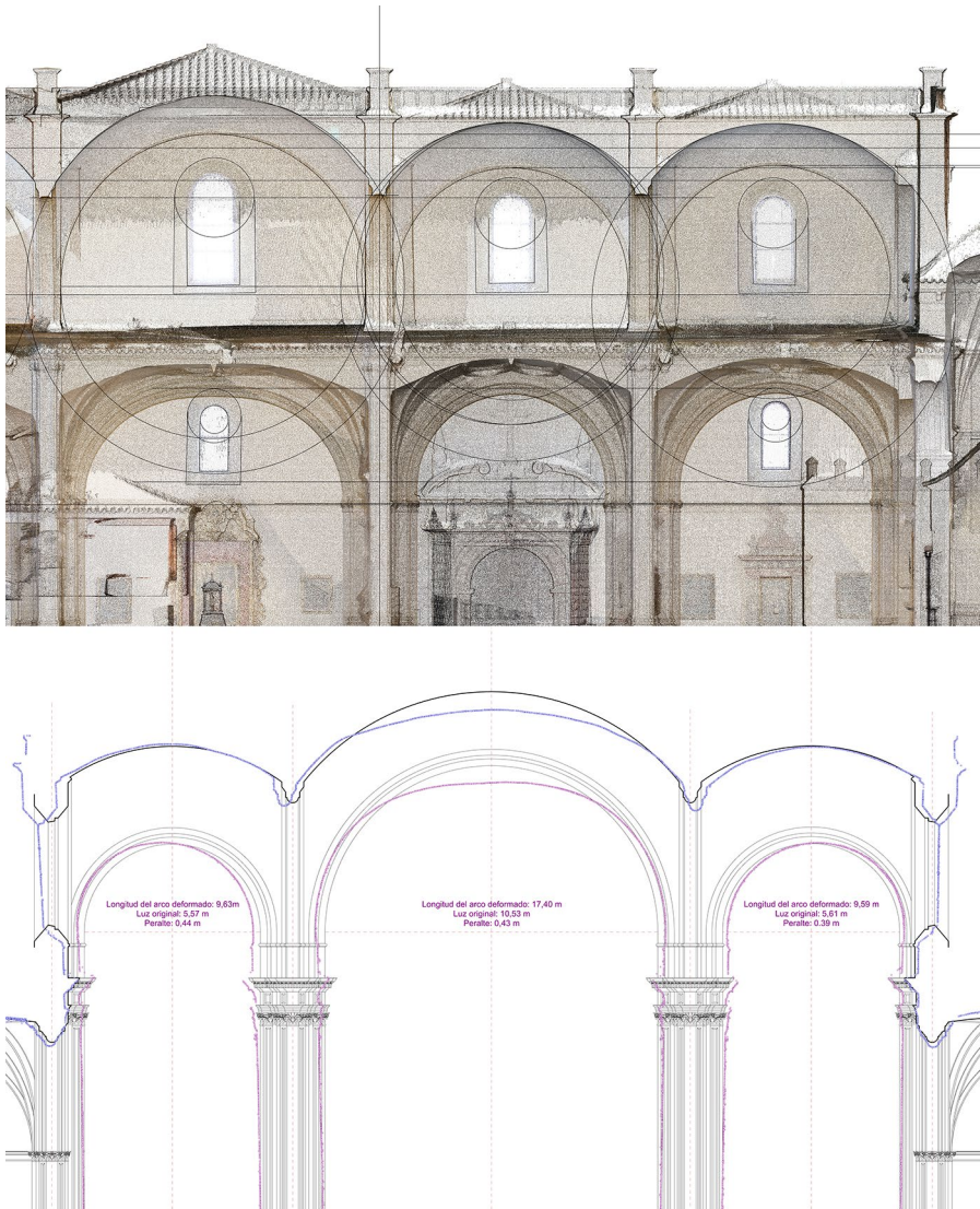
Fig. 8 Geometrisation of the point cloud and graphical reversion of the structural deformations
