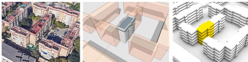
Fig. 7. Aerial view and energy models of the reference sample building in BEM and UBEM tools for the validation test.
