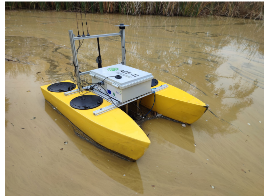
FIGURE 1. Example of an ASV prototype for the measurement of water quality parameters, equipped with GPS for path planning.
