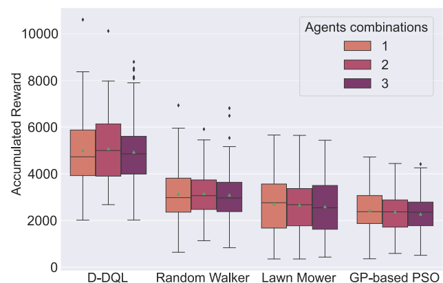
FIGURE 9. Box plot of the accumulated reward for the 3 combinations of agents according to the four algorithms compared during 100 episodes. The reward that would have been obtained by the algorithms that are not reward-driven is also computed, that is, heuristics other than DRL.
