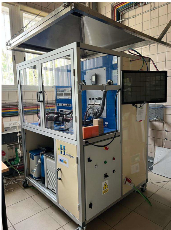
Fig. 9. PEM fuel cell test bench.
