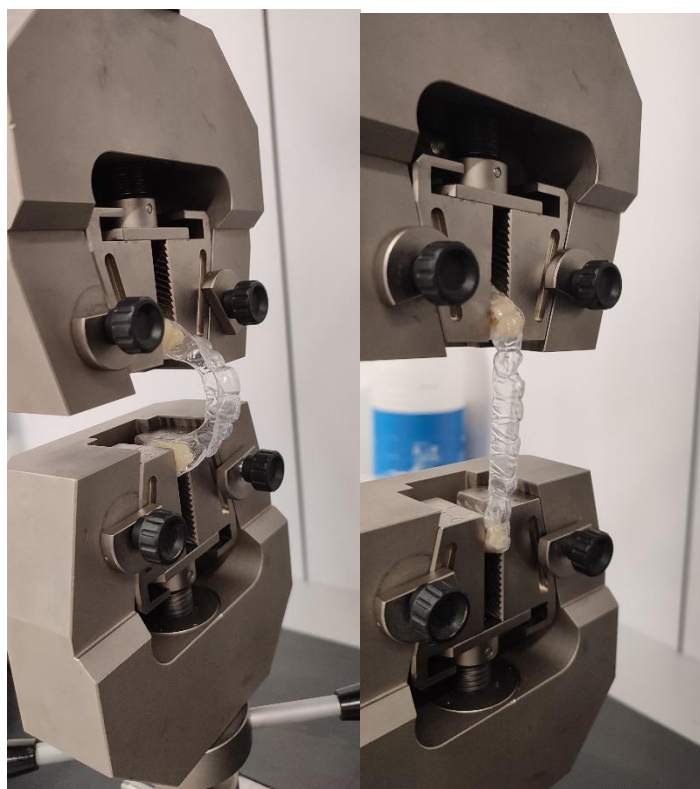
Figure 1. Stress–strain test for determination of mechanical properties.
