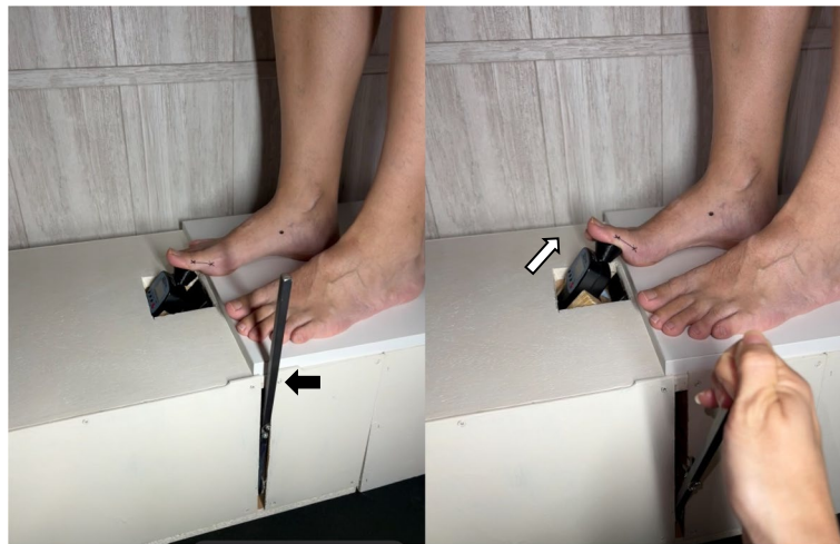
Fig. 2 Sequence of use of the digital force gauge used to perform the hallux dorsiflexion resistance test. The Pulley system (Black arrow) allows the digital force gauge to move upwards over the hallux (White arrow)
