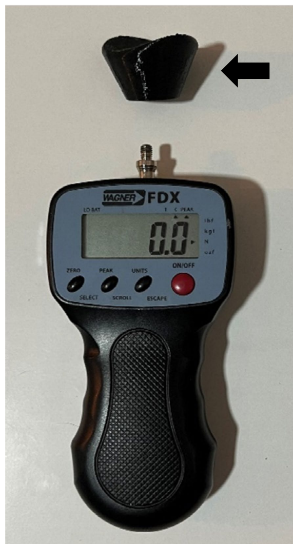
Fig. 1 Digital force gauge FPX ® 25 with a hallux adapter (Black arrow)
