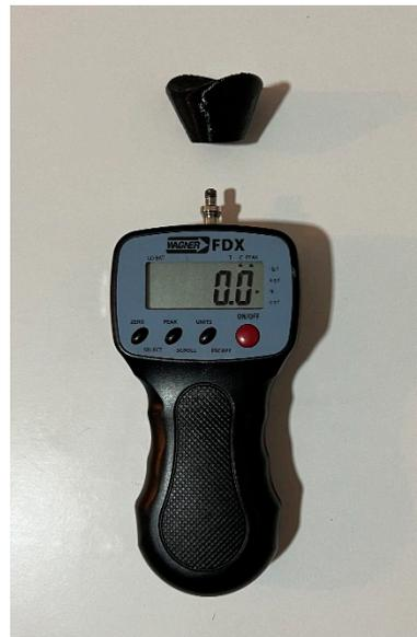
**Figure 1.** The digital force gauge with Hallux adapter (FPX<sup>®</sup> 25, Wagner Instruments<sup>®</sup>, Greenwich, CT, USA).
