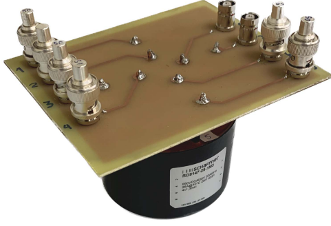
Fig. 17. 4W-CMC (SCHAFFNER RD8147-25-1M3) mounted on a PCB for measuring single-ended S-parameters with a two-ports VNA.
