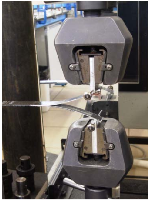
Figure 2.1: Interlaminar fracture toughness test set-up.
