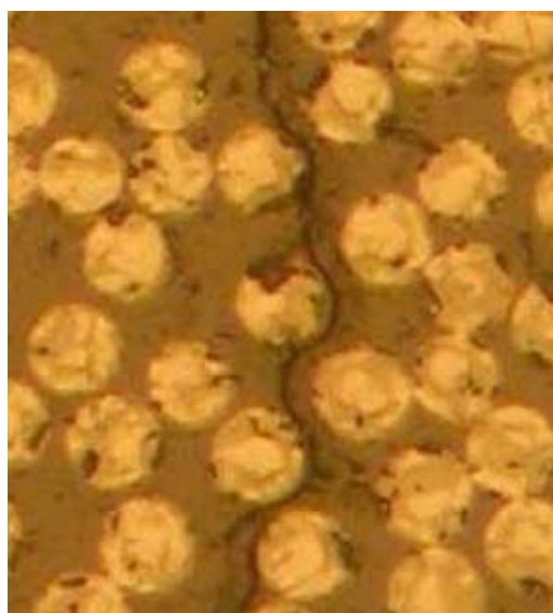
Figure 2.4: Damage in a composite material under tension transverse to the fibres. Taken from [46].
