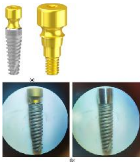
Figure 1. (a) Test implant and abutment (TEST); (b) Optical microscopy images of TEST implant (on the left) and Control implant (CTRL, on the right).
